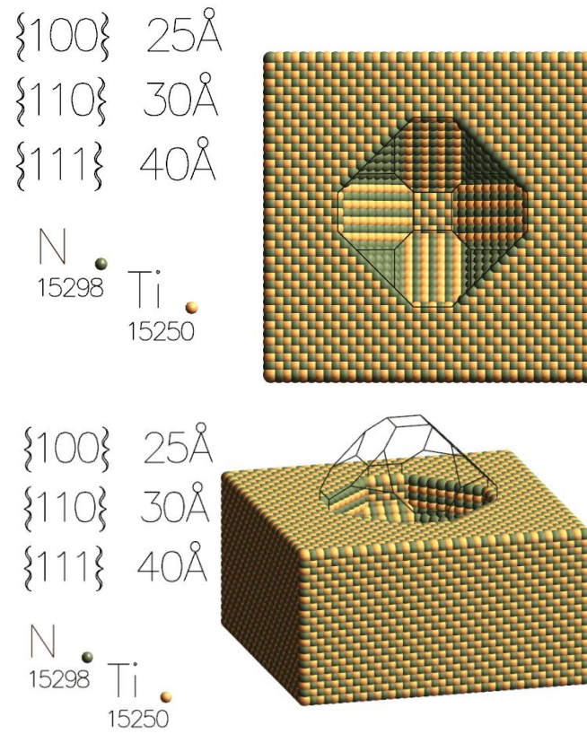
Figure 16: Vacuum on the (001) surface of the TiN Fm\bar{3}m crystal
