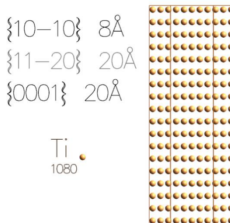
Figure 13: Ti P6_3/mmc constructed with the \{10\bar{1}0\} and \{0001\} families looking at the (10\bar{1}0) plane [8]
