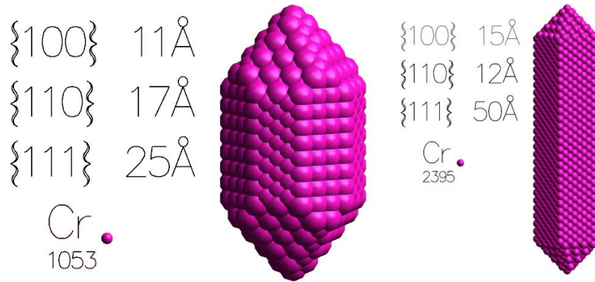
Figure 9: Rod-Like crystals, Cr Im\bar{3}m crystal [1]
